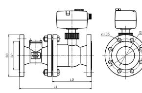
Above dimensions are for PN16 valve bodies. Please see the dimensions of actuator at data sheet of SBA05 and SBA06 actuator.
