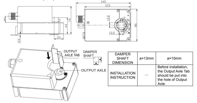
Note: Only suitable for  $13 \times 13$ mm or  $10 \times 10$ mm foursquare damper shaft. Other sizes of aluminum gaskets can be made when the Damper Shaft dimension "a" is smaller than 10mm.
