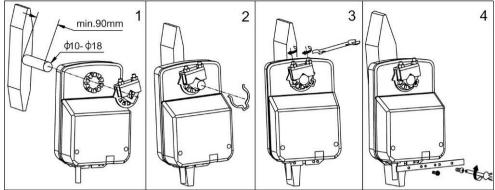
\* The accessories include 2 limitative baffles, 2 baffle setscrews (M3×6), and 1 actuator setting gasket.
